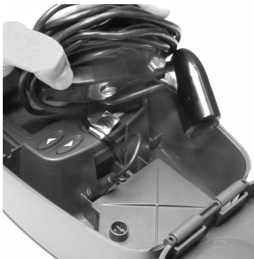
Stow transducer on top of battery cover.
